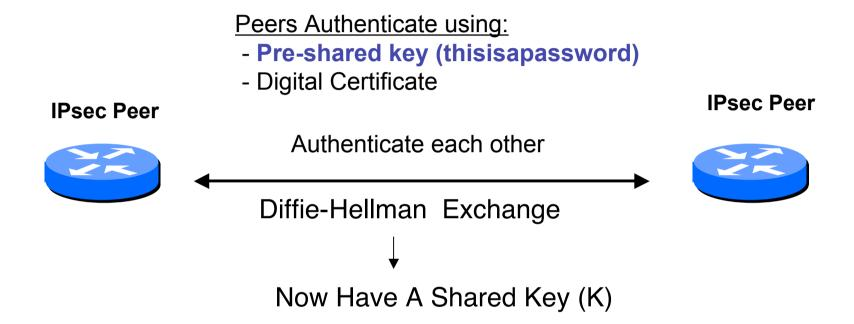
K is used to *derive* authentication key Authentication Keys get periodically re-created !!
