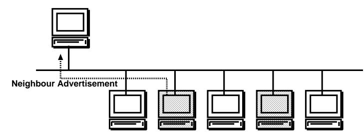
In most cases, solicited node multicast address includes only the target node
