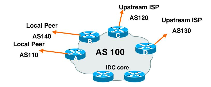
Assigned /24 from AS120 and /23 from AS130. Circuit to AS120 is 2Mbps, circuit to AS130 is 4Mbps
