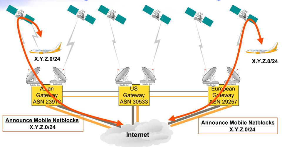
Commercial passenger traffic is released at each ground station Each ground station only advertises the IP's for the planes it is serving. When a plane leaves a region, that gateway stops advertising its IP's.
